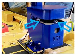
1. Scanner window must be protected from high pressure water, grease and dirt when cleaning the machine with high pressure equipment.
