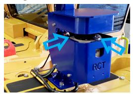
1. Scanner window must be protected from high pressure water, grease and dirt when cleaning the machine with high pressure equipment.
