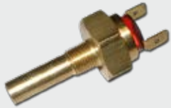
LIGHT DUTY TEMP SWITCH 100°C N/C THREAD: 1/8 NPT PART NO. 9454
