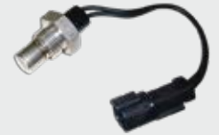
HEAVY DUTY TEMP SWITCH 107°C N/C THREAD: 3/4 UNO PART NO. 8491
