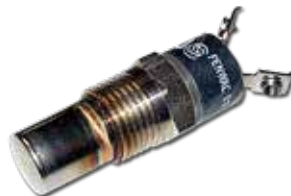
Part No: 2412 TEMPERATURE SWITCH 230°F NORMALLY CLOSED 2 SPADE TERMINAL 3/8NPT
