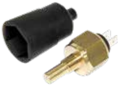
Part No: 11813 TEMPERATURE SWITCH 80°C NORMALLY OPEN 1/8NPT
