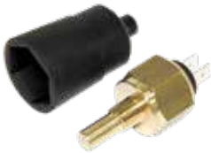
Part No: 11805 TEMPERATURE SWITCH 95°C NORMALLY OPEN 1/8NPT
