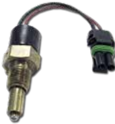
Part No: 6027 TEMPERATURE SWITCH 210°F 2 TERMINAL 3/8 NPT WEATHERPACK PLUG - NASON # TM-2A-210R/WP
