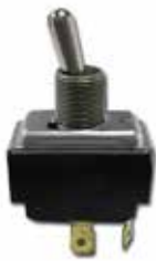
Part No: 7567 TOGGLE SWITCH ENVIRONMENTALLY SEALED ON - MOMENTARY OFF - SPADE TERMINALS
