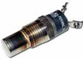
Part No: 1359 TEMPERATURE SWITCH 266°F NORMALLY OPEN 2 TERMINAL 3/8NPT
