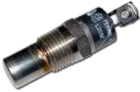
Part No: 1763 TEMPERATURE SWITCH 205°F NORMALLY CLOSED 2 TERMINAL 3/8NPT
