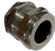
Part No: 2698 METAL GLAND 25MM 14.5 - 20.5MM DOME TOP
