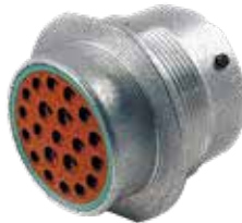
Part No: 0930 RECEPTACLE MALE HD34 - 21 PIN - 4 X #12, 17 X #16 CONTACT DEUTSCH # HD34-24-21PN
