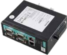
Part No: 14655 MOXA RS232-ETHERNET SUITS AAC ANALOGUE
