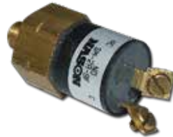
Part No: 3430 PRESSURE SWITCH 9PSI FALLING 1/8NPT NORMALLY OPEN
