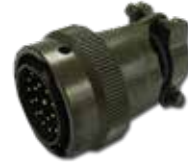
Part No: 0184 CABLE MOUNT FEMALE BAYONET 23 PIN SIZE 16 SHELL MS3116S16-23P
