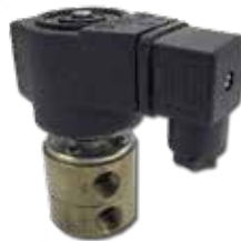
Part No: 9071 AIR SOLENOID VALVE 24V 3 PORT NORMALLY OPEN - DIN PLUG
