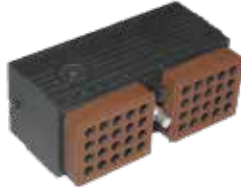
Part No: 6706 PLUG FLANGED DRC 10 - 40 PIN MOULDED CONTACTS DEUTSCH # DRC10-40-P
