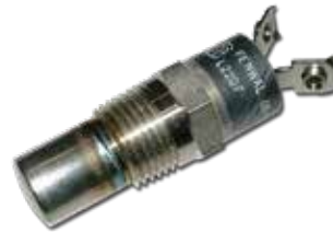
Part No: 1765 TEMPERATURE SWITCH 220°F NORMALLY CLOSED 2 TERMINAL 3/8NPT
