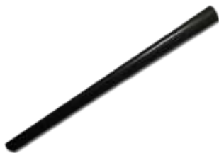
Part No: 5075 HEATSHRINK RESIN LINED DUAL WALL 19 - 6MM BLACK
