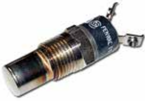
Part No: 7168 TEMPERATURE SWITCH 300°F NORMALY CLOSED 2 TERMINAL 3/8NPT
